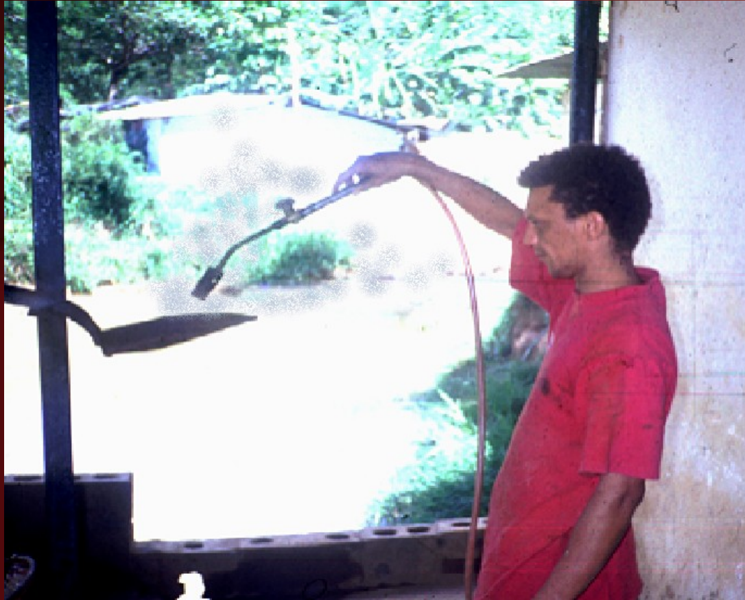
Venezuelan miner burning amalgam in a shovel and inhaling mercury vapor
