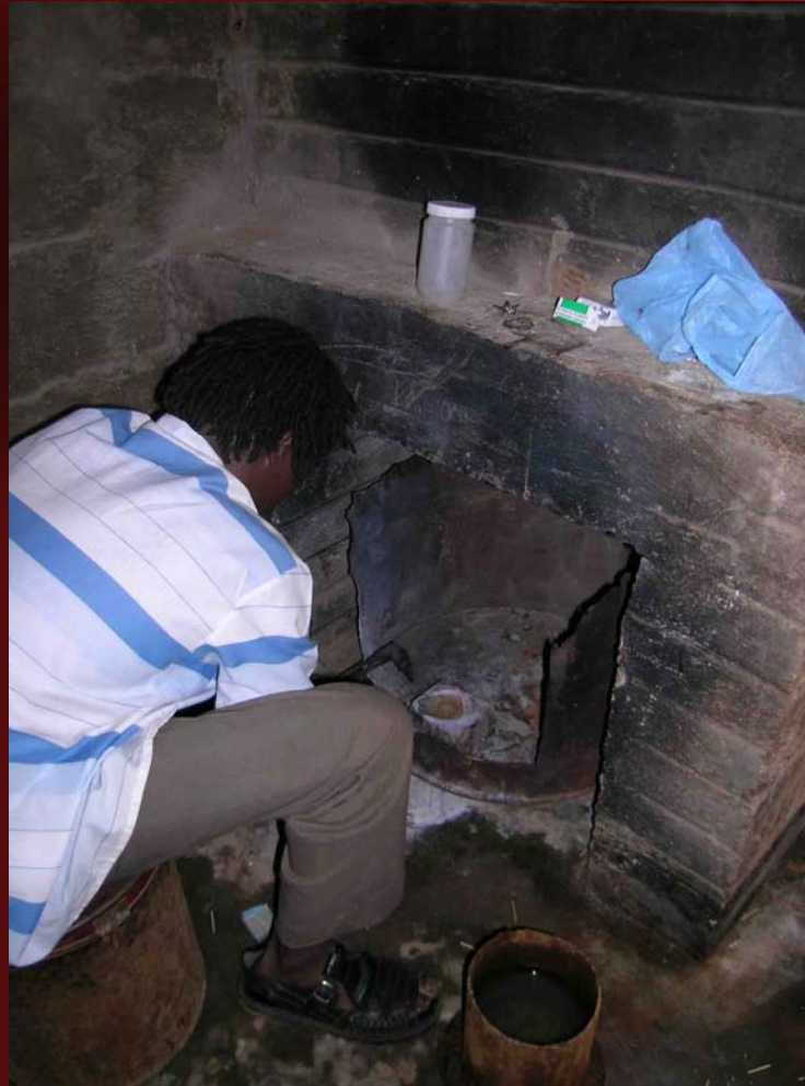
Demonstration of burning off mercury from mercury/gold amalgam ball
